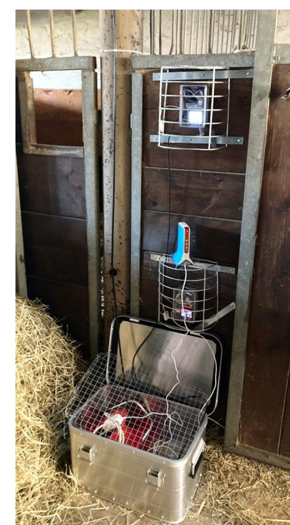
Fig 1 Dust SDS011 sensors 50 cm and 120 cm in the box
