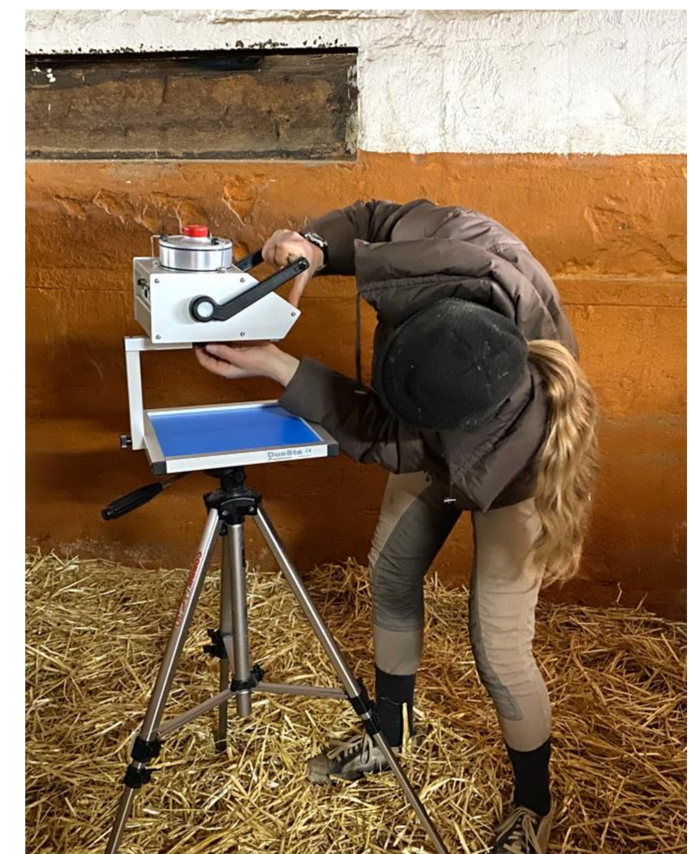
Fig 2: Air sampling system (MBASS30v3, Holbach GmbH)
